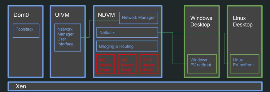
Default configuration: All of the physical PCI network devices are assigned to a single Network Device Virtual Machine (NDVM) and isolated using VTd.
